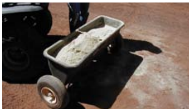
Above, a rototiller on a 3-point tractor hitch makes an effective mixing implement. Below, an adjustable spreader box towed behind an ATV was used to measure out bentonite clay. The clay was too fine and the spreader box did not work well.
