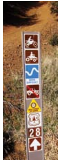
These signs have too much information and the important information like trail number and direction are not at the top where they should be. Agency and funding decals, if needed, should be at the bottom of the marker. Riders will not stop long enough to read or comprehend this data.
