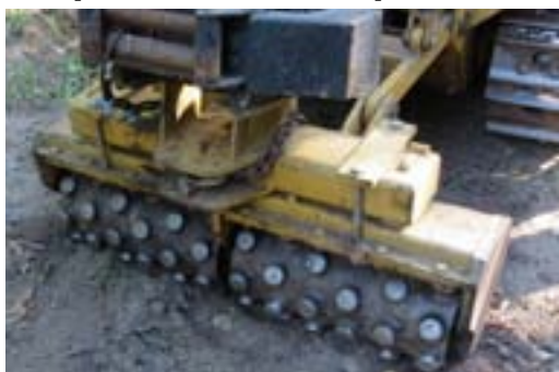
This sheep's foot roller attachment behind a trail dozer doesn't vibrate, but it does a good job of compaction when there are favorable soil moisture conditions.
