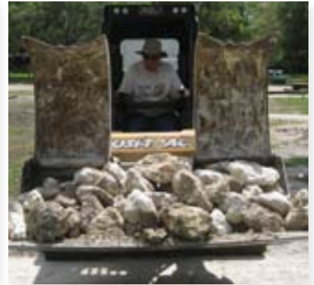
If one thumb is good, two has to be better. A clamshell bucket can hold material with odd shapes and sizes.
