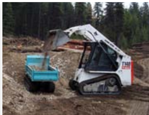
Whether used as loaders or haulers, skid steers are versatile trail-sized equipment. Because they are tracked with low center of gravity and good braking ability, they are far more stable and safer as a tow vehicle than an ATV or ROV.
