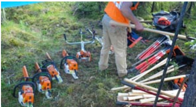
It can be challenging just getting the tools and gear to the work site. From L to R, chainsaws, brush cutters, shovels, McLeods, pulaskis, and loppers.
