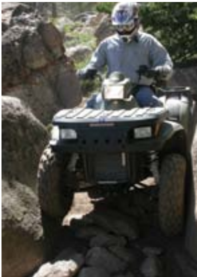
Here the tread is so narrow that riders must put a tire up on the rock on the left to get through. This can tip the vehicle toward the right which increases the risk of a bent rim, a broken bead, and scratched or broken plastic.
