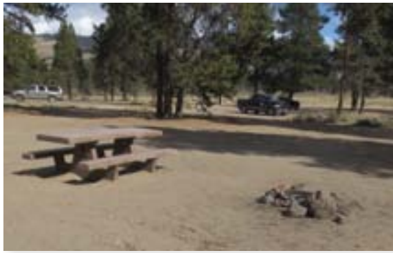
Concrete picnic tables are durable and they deter theft, but the shade moves and they don't. With no shade and smoke from the fire drifting toward the table, will it get used?
