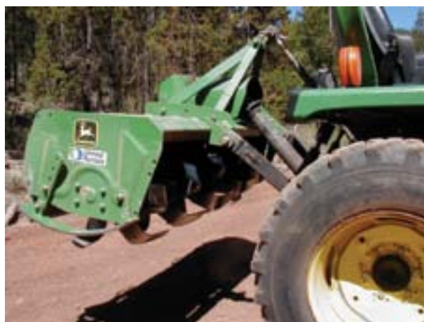
Above, a rototiller on a 3-point tractor hitch makes an effective mixing implement. Below, an adjustable spreader box towed behind an ATV was used to measure out bentonite clay. The clay was too fine and the spreader box did not work well.
