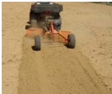
The rock rake can cut material from the edges and drift it into the center. Combs are available in different widths. At full tilt, this fixed comb extends past the width of the ATV to retrieve berms.
