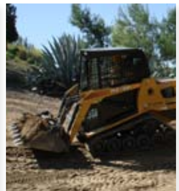
Whether used as loaders or haulers, skid steers are versatile trail-sized equipment. Because they are tracked with low center of gravity and good braking ability, they are far more stable and safer as a tow vehicle than an ATV or ROV.
