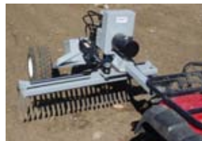
This sliding comb rake can reach out and retrieve material that is normally unrecovered and wasted in berms.
