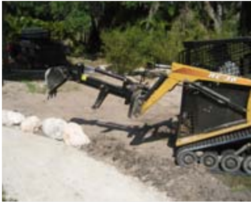
The wide range of attachments for skid steers makes them useful for a variety of tasks. This bucket attachment with a fixed thumb works well for placing these barrier rocks.
